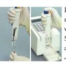
Draw the sample and reference solution with the Twin-pipette. Set the pipette and apply.
